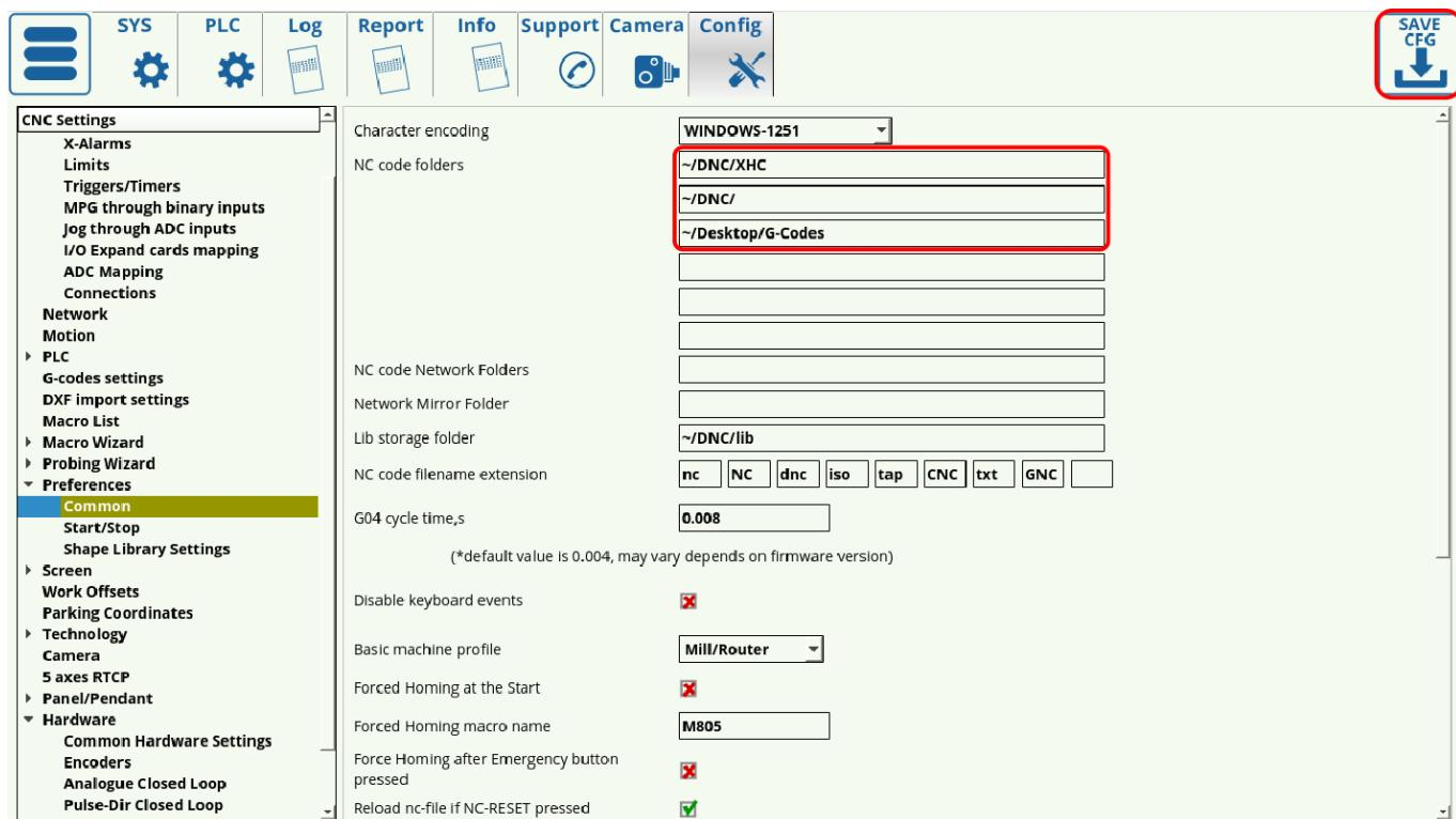
The screenshot shows the 'CNC Settings' configuration page in the myCNC software. The 'NC code folders' section is highlighted with a red box, containing the paths: ~/DNC/XHC, ~/DNC/, and ~/Desktop/G-Codes. A 'SAVE CFG' button is located in the top right corner of the interface.
