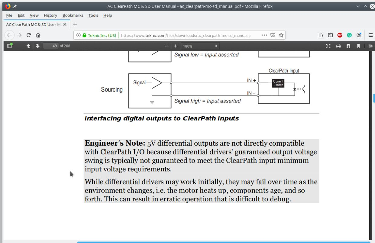
Effectively, a converter board is necessary to create a steady 5V signal which the ClearPath driver will be able to register. These line driver to 5V converter boards are available as part of certain kits on the myCNC [Online Shop](#).
