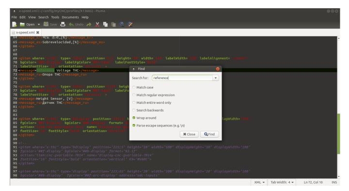
• It can be seen that the Proc and THC Speed labels are located in the x-reserv section, while the Reference Voltage THC and Height Sensor are situated in the x-thc section (this can be seen in the "where="field" field). We will condense the existing labels and display elements
