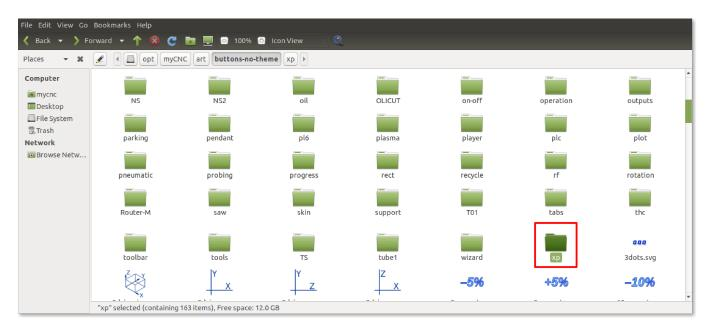
• The two buttons that will be used to turn the gas on and off currently do not have their respective images. These will be added to the gas folder within the xp theme folder described above. They will be called button-gas-on.svg and button-gas-off.svg respectively. The images are created using a program capable of making an .svg file, like Inkscape (free, open-source vector graphics application).
