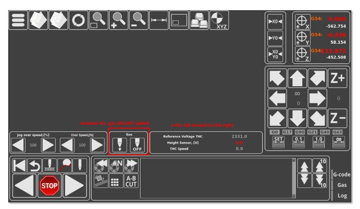
As can be seen in the screenshot above, the program now has two new on-screen buttons for gas on/gas off, as well as having the previously available information condensed into relocated x-thc tab.
