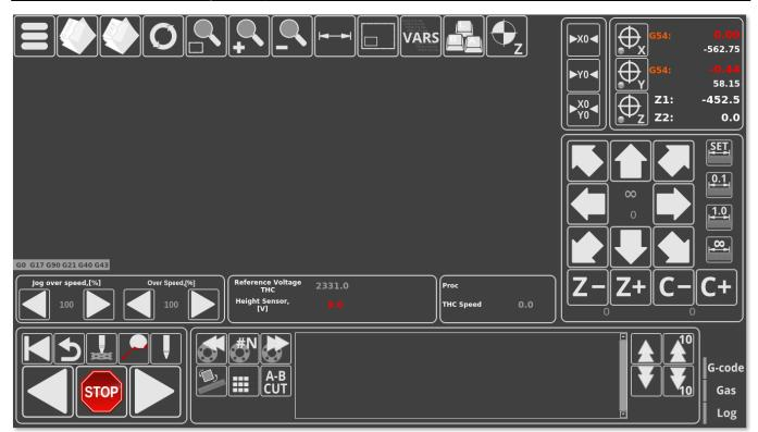
• The new buttons need to be inserted into some space on the main screen, so that they are easily accessible. No such readily available space exists on the screen at this point, so it has to be created. It has been noted that the functions in the two tabs next to the overspeed / jog overspeed buttons can be condensed into one tab.
