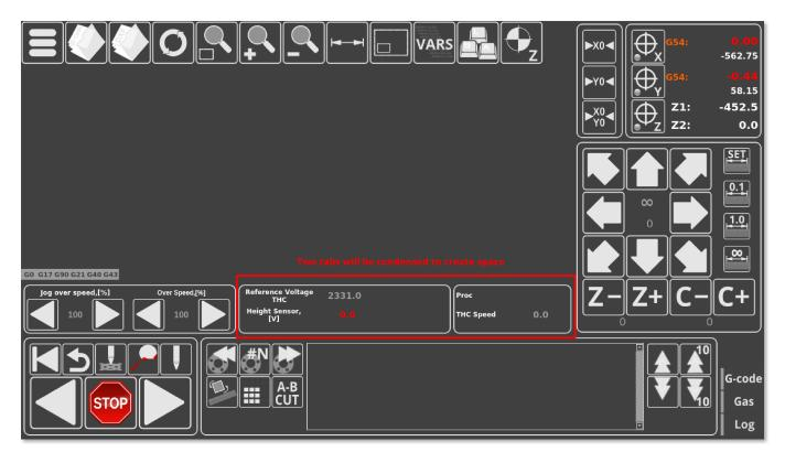
In order to condense these tabs, we have to head into the config files for the myCNC application. Go to your Home folder, the navigate to .config/myCNC/profiles/X1366G. In this folder, locate the x-speed.xml file and open it in the text editor of your choice (Pluma was used in this example). Note that different sections of the screen and different tabs can be described in different .xml files within the profile folder. What brings them all together is the
