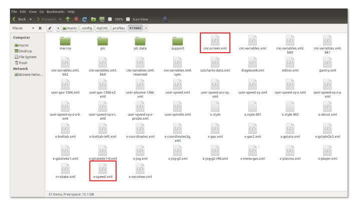
In the x-speed.xml file, navigate to the section that describes the two tabs which will be condensed (the easiest way to do so would be to use the Ctrl+F function to search for the labels used within these tabs such as "Reference Voltage")
