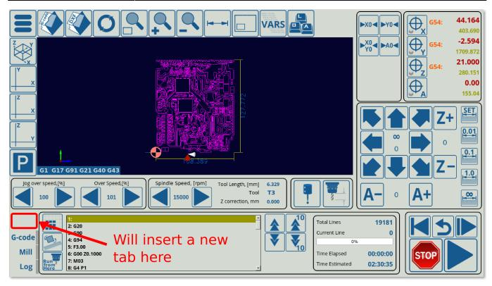
• The code for the bottom tab can be found in the x-bottab-left-mill.xml file in the main profile folder (X1366M4). This file should be specified in the cnc-screen.xml file, to indicate to the program that this code will be included on the main screen. The line in the cnc-screen.xml file should look the following:
