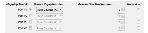
Next, you must select the counter number to which the sensor is connected. The number of the counter depends on the version of the controller, so please refer to the controller documentation for the correct definition of the counter number.
