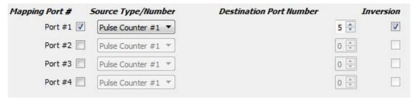
If it is necessary to invert the value of the sensor, simply check the check box for the desired inversion. Inversion can be useful if, for example, the value from the sensor increases as the distance decreases, but it is necessary that the value of the sensor decreases when the distance is changed.
