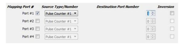
Next, select the virtual channel number of the ADC, in which the counter value will be placed in the register. Virtual channels begin their numbering right after the numbers of real ADC channels. le if you have on the controller for example four channels of ADC (ADC0, APC1, APC2, APC3), then the first channel number will be ATSTS5 and you accordingly need to select channel number 5.
