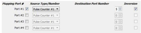
5. For tracking, it is more convenient if the value of the ADC register increases with increasing distance to the object, and decreases when you approach the object. Our sensor works the other way around. Therefore, set the inversion on the selected port.
