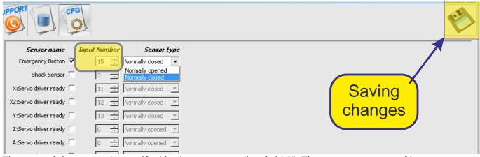
The type of the sensor is specified in the corresponding field "". There are two types of input sensors.
