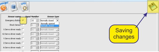
The input number on the controller board is set in the corresponding field "Inputs Number" Numbering of inputs can be found in the documentation for the selected window controller.
