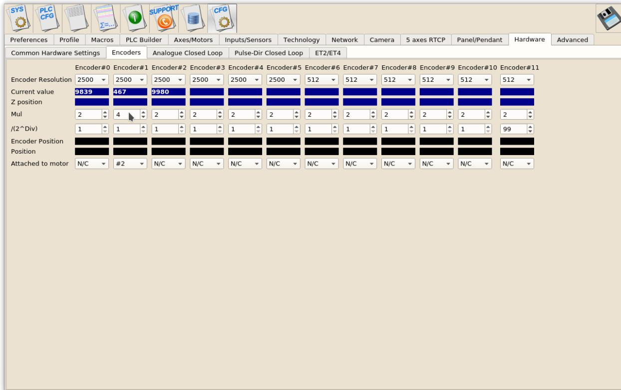
2. Set **Mul** and **/(2^Div)** ratios to get result Encoder resolution equal to **Pulses-per-Unit** resolution. For example
