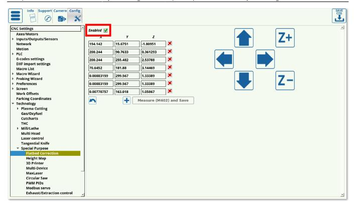
Next, the table on the settings page presents a number of values in the XY-plane and their z-positions. These values can either be inputted manually by using a sensor and recording the position by hand, or by using the M402 macro. In order to use the macro, move the sensor to the position you want to measure, then press the **Measure (M402) and Save** button. This will lower the sensor down until contact, then lift it back up and record the z-position at which the sensor was triggered.
