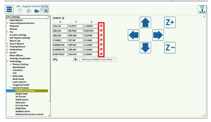
By adding these correction points, myCNC software will use triangulation in order to create a complete updated map of the working table. From here on, whenever Flatbed Correction is enabled, the machine will automatically adjust the z-axis height of the working tool in order to adjust for the table level changes depending on where in the XY-plane it currently is.
