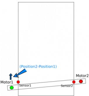
6. Then, after the alignment has completed the second motor control is activated again and both motors will be moving together to move out by the set distance
