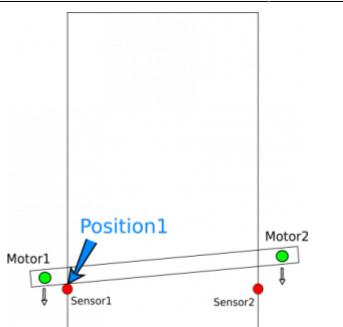
3. Motion is stopped at the moment both sensors are triggered.
