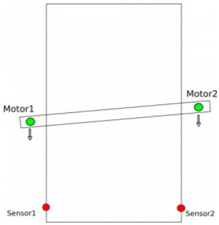
2. When one of the sensors is triggered, CNC control disconnects the motor on that side, while the second motor continues to move.
