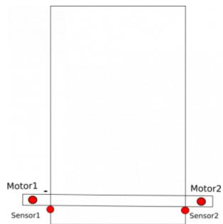
4. It is important to note that the sensors do not have to be perfectly aligned on the same line they can be placed wherever it is convenient, provided that the offset distance between them is accounted for in the Tuning field:
