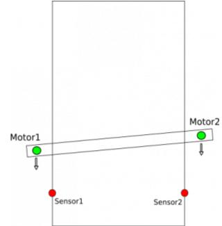
2. PLC controller procedure records machine positions at the moment that each respective sensor is triggered.
