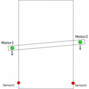
2. When one of the sensors is triggered, CNC control disconnects the motor on that side, while the second motor continues to move.
