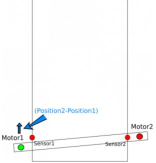
6. Then, after the alignment has completed the second motor control is activated again and both motors will be moving together to move out by the set distance
