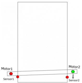
3. When both sensors are triggered, the motion stops.
