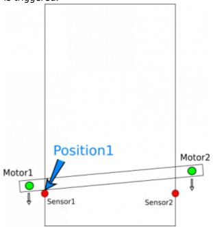
3. Motion is stopped at the moment both sensors are triggered.
