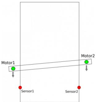
2. PLC controller procedure records machine positions at the moment that each respective sensor is triggered.
