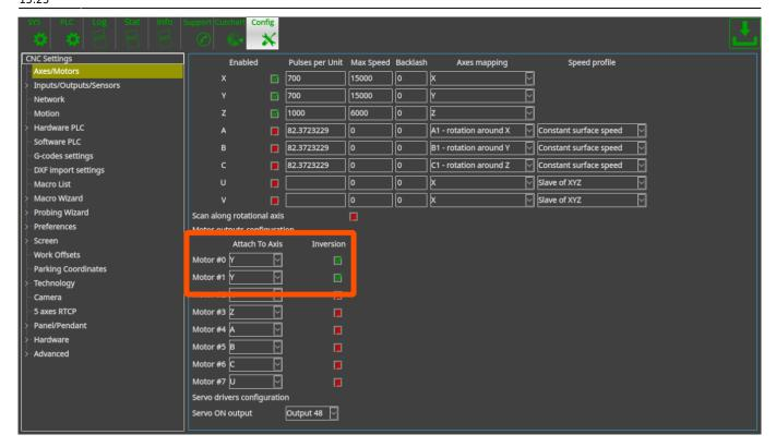
2) Procedure to connect both outputs to Y axis will look the following:
