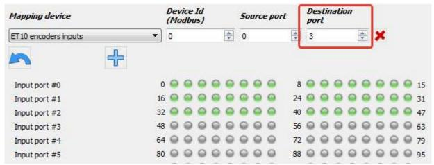
• This example shows how to connect an external controller to the modbus interface. At the remote controller with id = 1 input port number 2 (inputs from 32 to 47) is pushed to the input virtual port of controller number 3 (inputs from 48 to 63)
