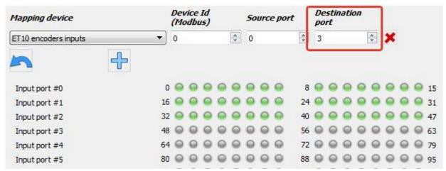
• This example shows how to connect an external controller to the modbus interface. At the remote controller with id = 1 input port number 2 (inputs from 32 to 47) is pushed to the input virtual port of controller number 3 (inputs from 48 to 63). The LED layouts below show the state of the port for each of the inputs.
