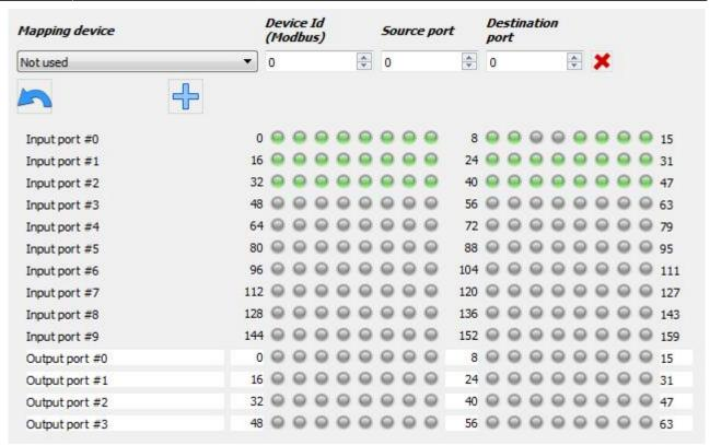
• Next, select the redirection conditions and the register for the mapping
