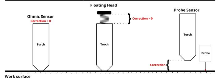
After the contact has been made, the machine will travel up by the IHC Ignition Height + the IHC Correction Height:
