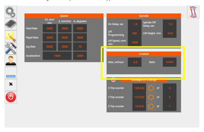
The programming of Pulse the Coolant widget is shown below.
