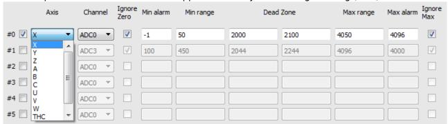
• It is also necessary to choose the number of the ADC input channel on the controller, where the analog signal from the analog control (analog-joystick) will go directly.
