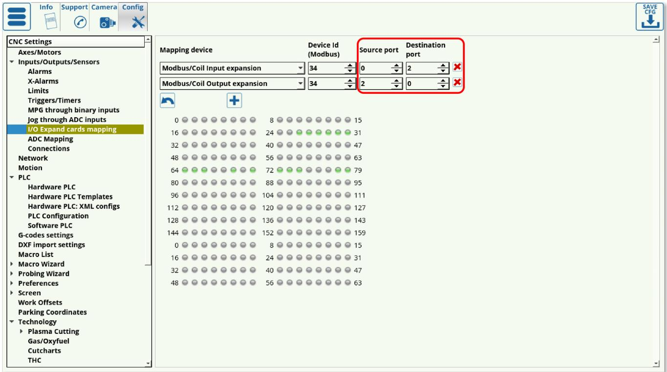
This inversion results from the Source and Destination being effectively flipped when using input/output ports via a Modbus. With inputs, the source is the Modbus device, while with Outputs, the source is the host computer/controller.
