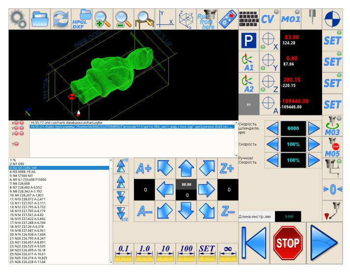
To start new job A position should be roll back to about "0" position. Jogging to "0" may take a long time (can be hundreds of complete turn to run). In some cases it's possible just reset A position, but A axis orientation will be lost. The best way to subtract a number of complete turns (360 degree), then move to "0" for the rest of A.
