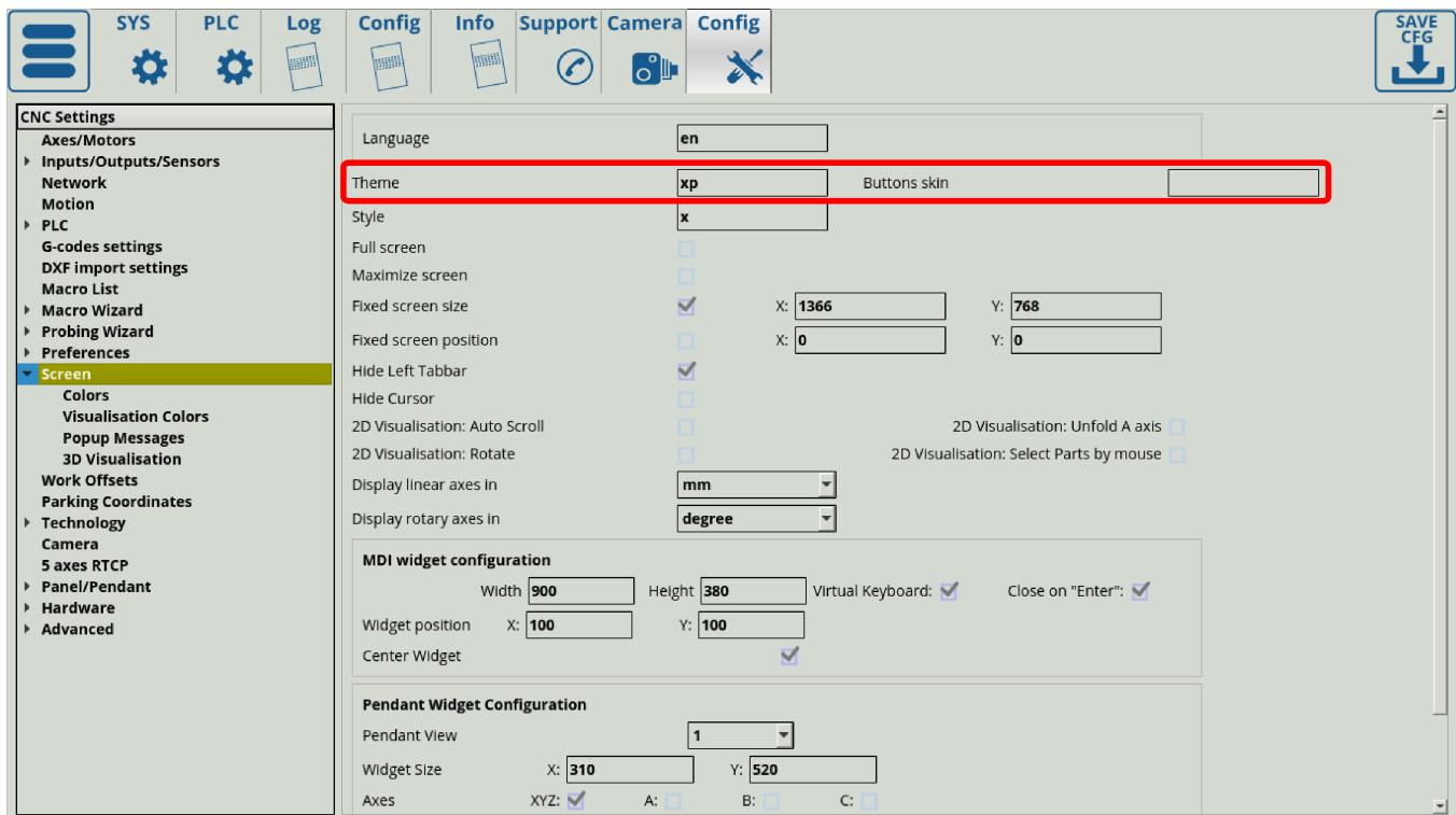
By default, the **xp** theme is used for the 1366 series profiles to insert images for buttons and display elements. You can read more about screen editing in the [MyCNC Screen Configuration](#) manual.
