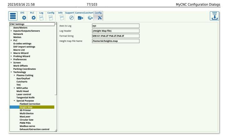
The height map is typically utilized for the per-job height probing described in the 3D Height Mapping manual. It is necessary to change the filepath to include the correct username for the machine (for example, /home/USERNAME/heights.map) as opposed to the default username specified in myCNC software (sk/mycnc/etc).
