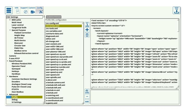
This window lists all the relevant profile xml files which define how the screen, settings, etc are laid out. These files should not be edited unless strictly necessary, as it they define the entire screen layout, the current settings config, the tools, and more.
