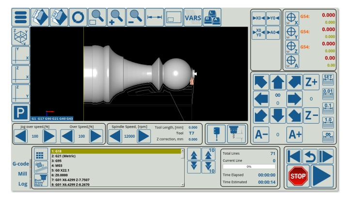
• Render time limit. On slower machines, such as TinkerBoard computers, it is often recommended to set a low time limit (2-5 seconds) to not overwhelm the system. The program will still run despite the visualization not being loaded all the way through.
