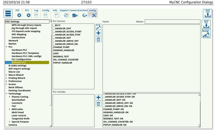
The Software PLC list consists of the PLC macros such as the Oil Change Counter and the Popup Handler which are done on the software side, rather than the hardware side. These Software PLC commands typically consist of items which are less time-critical, but require a continuous timer (like the oil change counter), or items which are loaded once the software is started/existed (<u>HANDLER INIT and HANDLER EXIT</u>).
