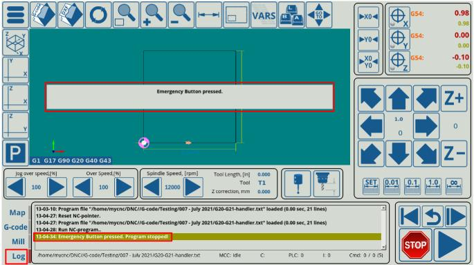
To configure the input port that will be assigned to the Emergency Stop button, please enter the necessary port value in Settings > Config > Inputs/Outputs/Sensors > Alarms. An example of Emergency button configuration is shown in the picture below:
