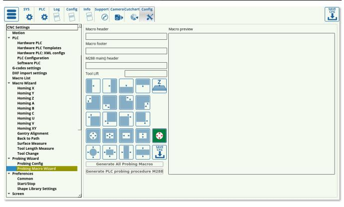
This wizard involves the macro header, the macro footer, the main() header for the automatically generated M288 macro, the necessary tool lift to safely move the probe over to the required location, and the available shapes for each of which a different macro can be generated (the macro names can be seen in the top line of each respective shape macro). These shapes allow to load in a macro preset for the particular case, and to easily edit the probing macros.
