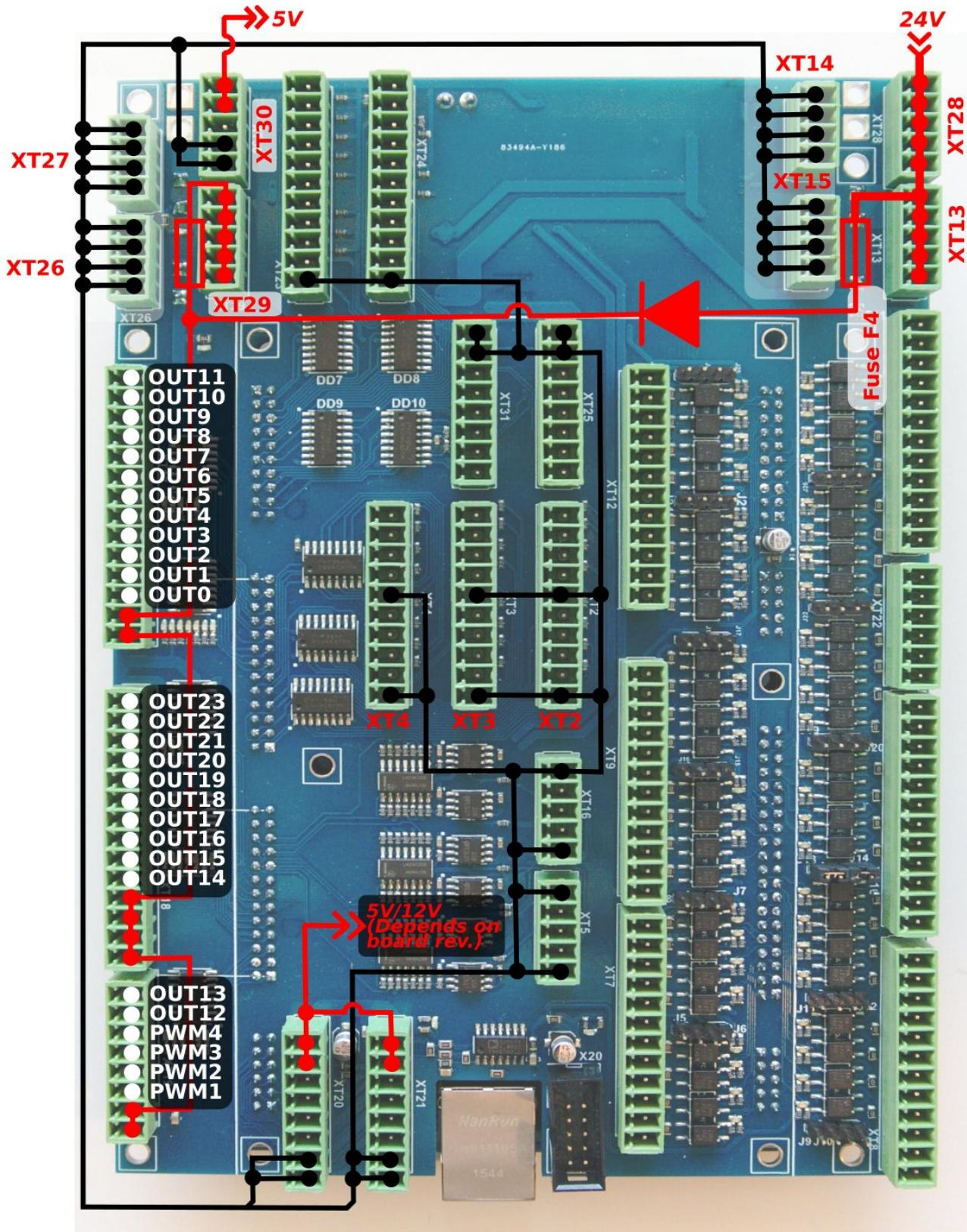
There are LED indicators for each Output pin on the ET10 board to control actual Output state. LEDs are highlighted in a picture below.
