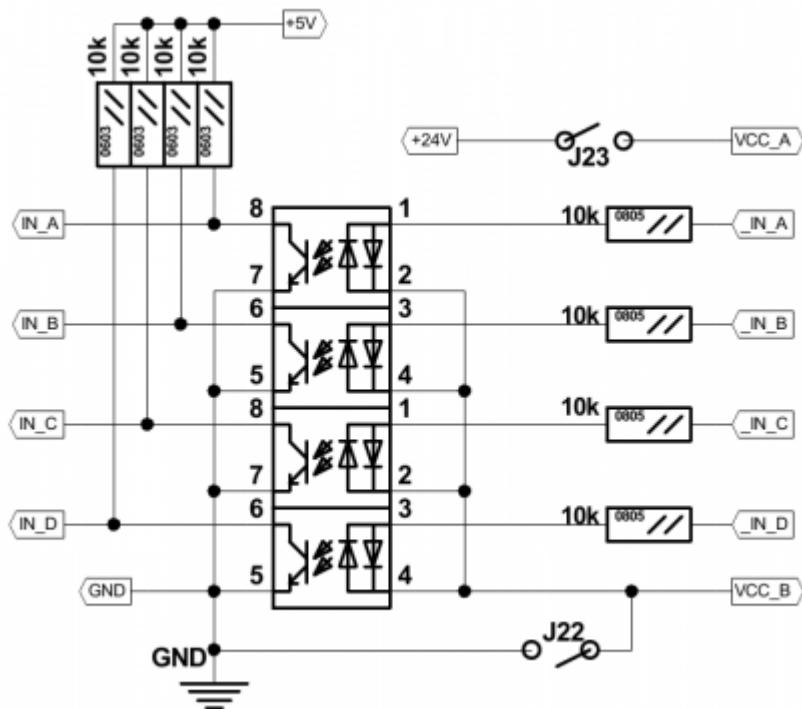
Wires VCCB(common wire) and VCCA are used for external power supply connection. Beside external power supply, internal +24V DC can be used to supply input LEDs, if correspondence jumpers are closed.
