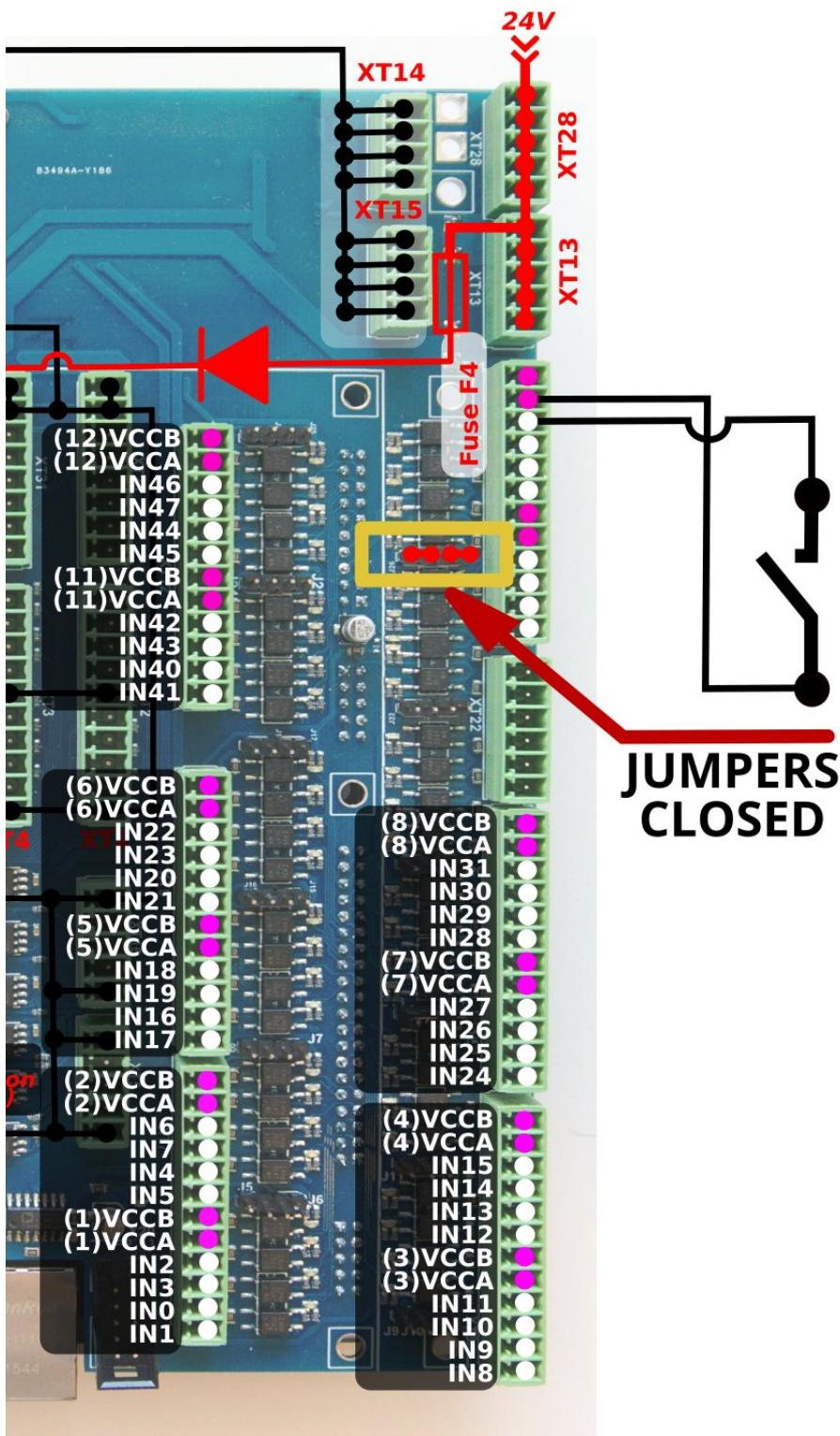
Common wire for 4 optocoupler units is connected to internal GND (0V) if the Jumper is closed. A switch should short another optocoupler input to +24V to activate input pin.
