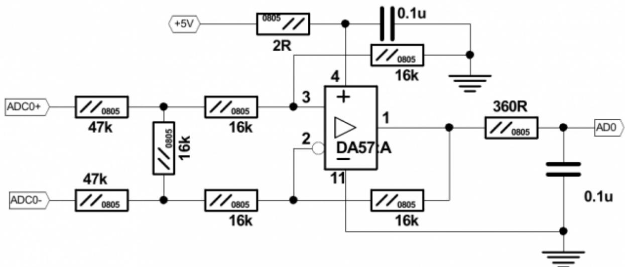
Input schematic for ET10 0-5V ADC inputs (Channels#1...#7)
