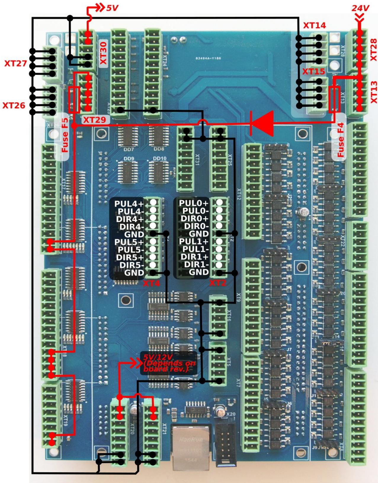
PULSE-DIR channels 2,3 pinout
