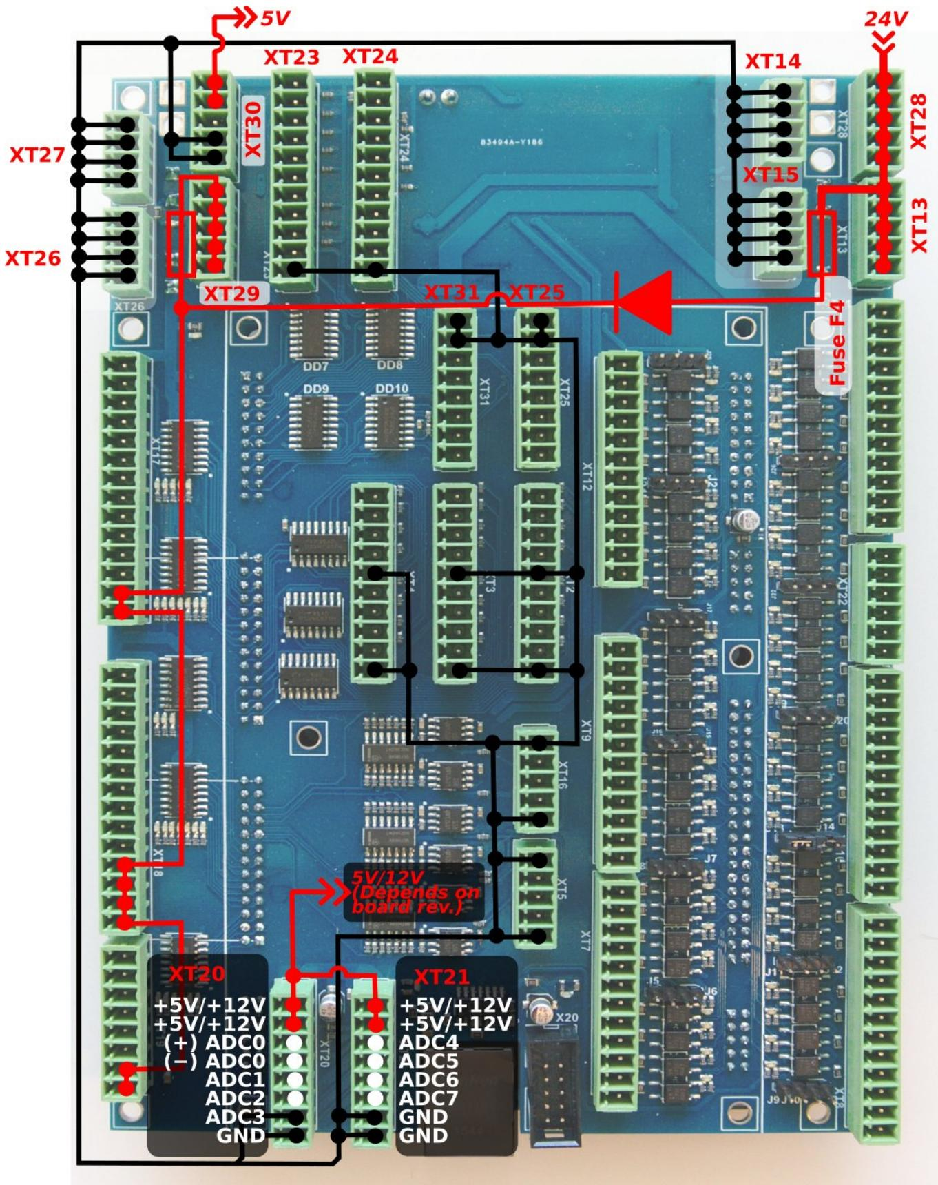
The picture below shows an example of a potentiometer connected to ADC2 input.
