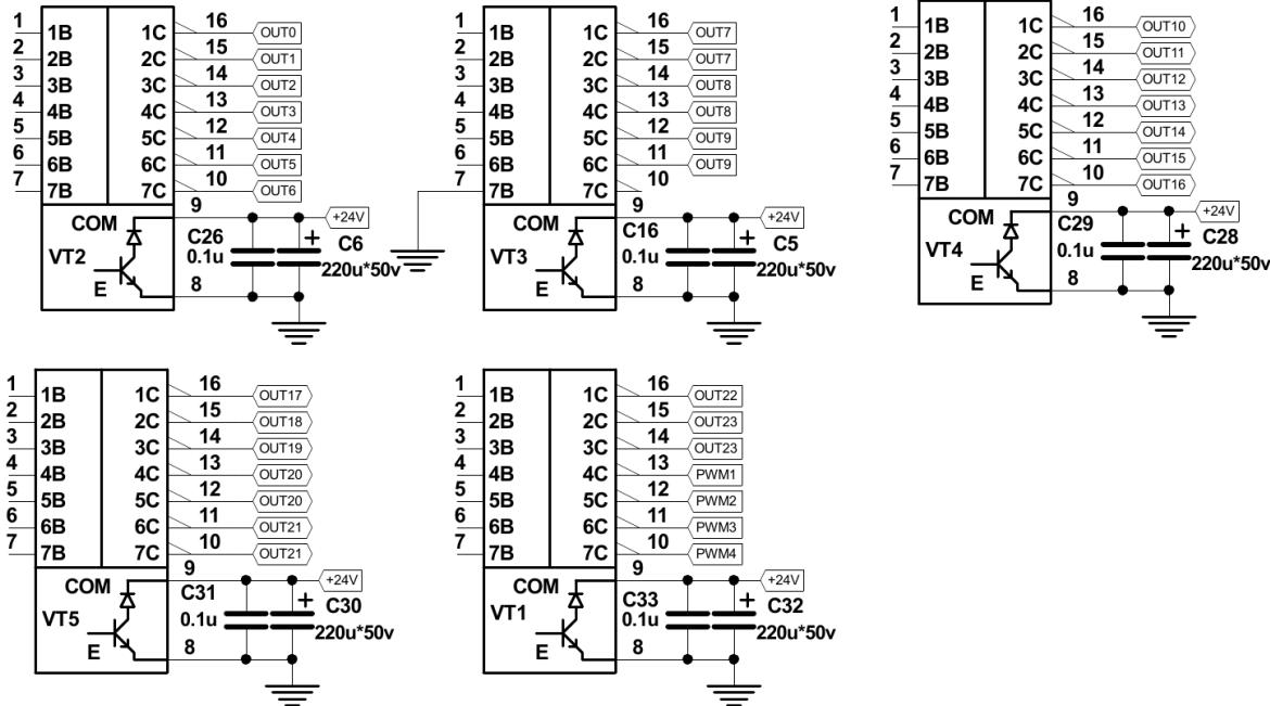
ET10 pinout for outputs is shown below
