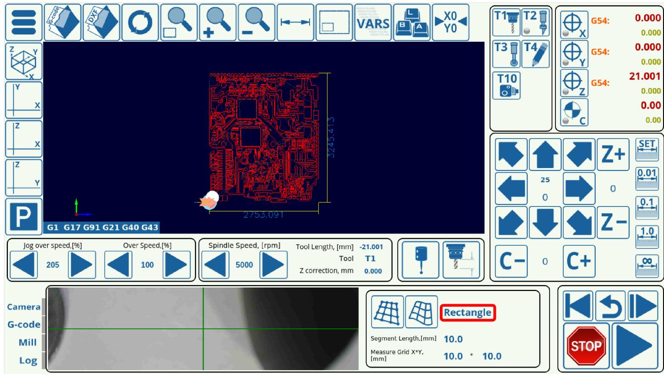
If we look at the code, the RadioDisplay element is actually using the cnc-gvariable-toggle to change between the two modes (0 for Rectangle, 1 for Area):
