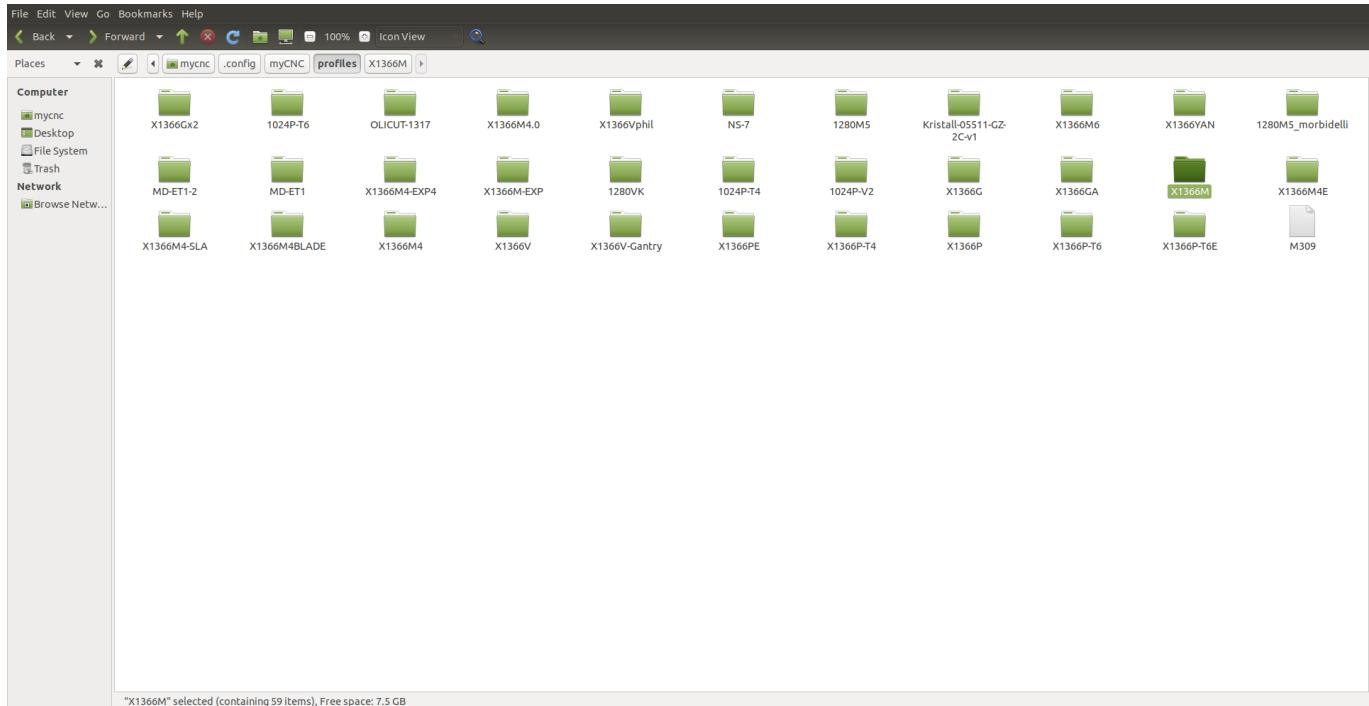
Upon opening the necessary profile folder (we will be using X1366M in this example, for the simple 3-axis mill profile), you are presented with a list of all the .xml files which will populate your screen:
