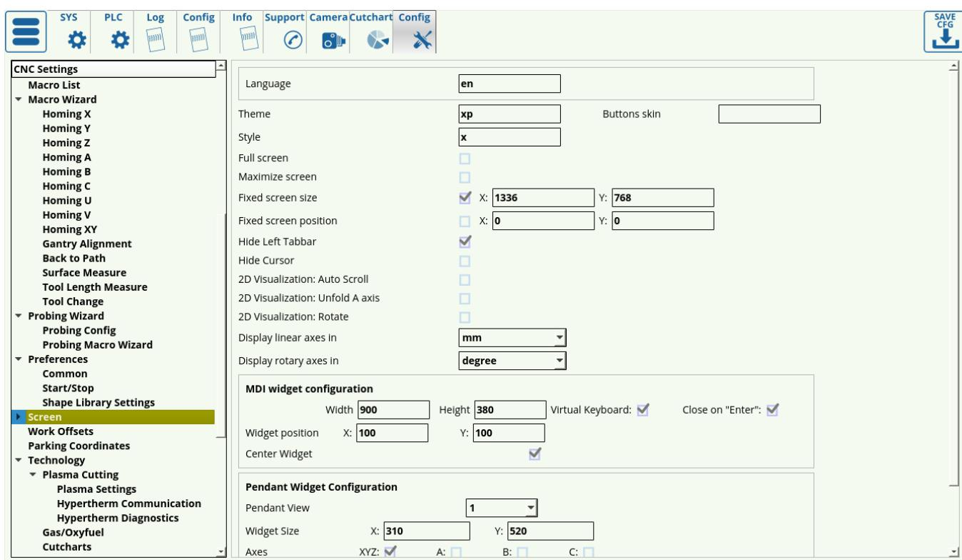
The “x” is the default on all modern myCNC profiles, with the `x.style` customization file located in the profile folder ([MyCNC profiles](#)). Editing this file allows for deeper customization of certain on-screen elements that are typically left to their default configuration (such as radio buttons, spinboxes, and other low-level GUI elements).
