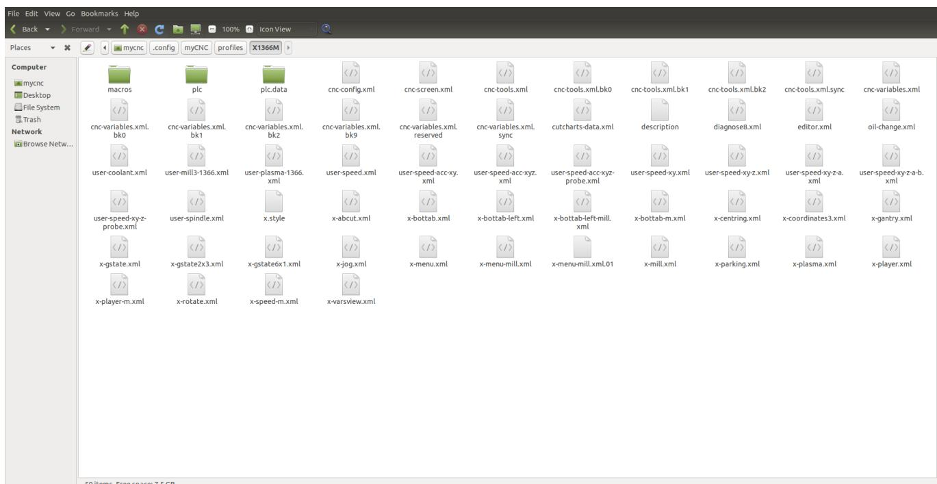
However, merely being in the profile folder does not mean that the .xml file's contents will be displayed on the myCNC screen. In order for the .xml file to be used, it must be included in the cnc-screen.xml file that is located within that profile's folder:
