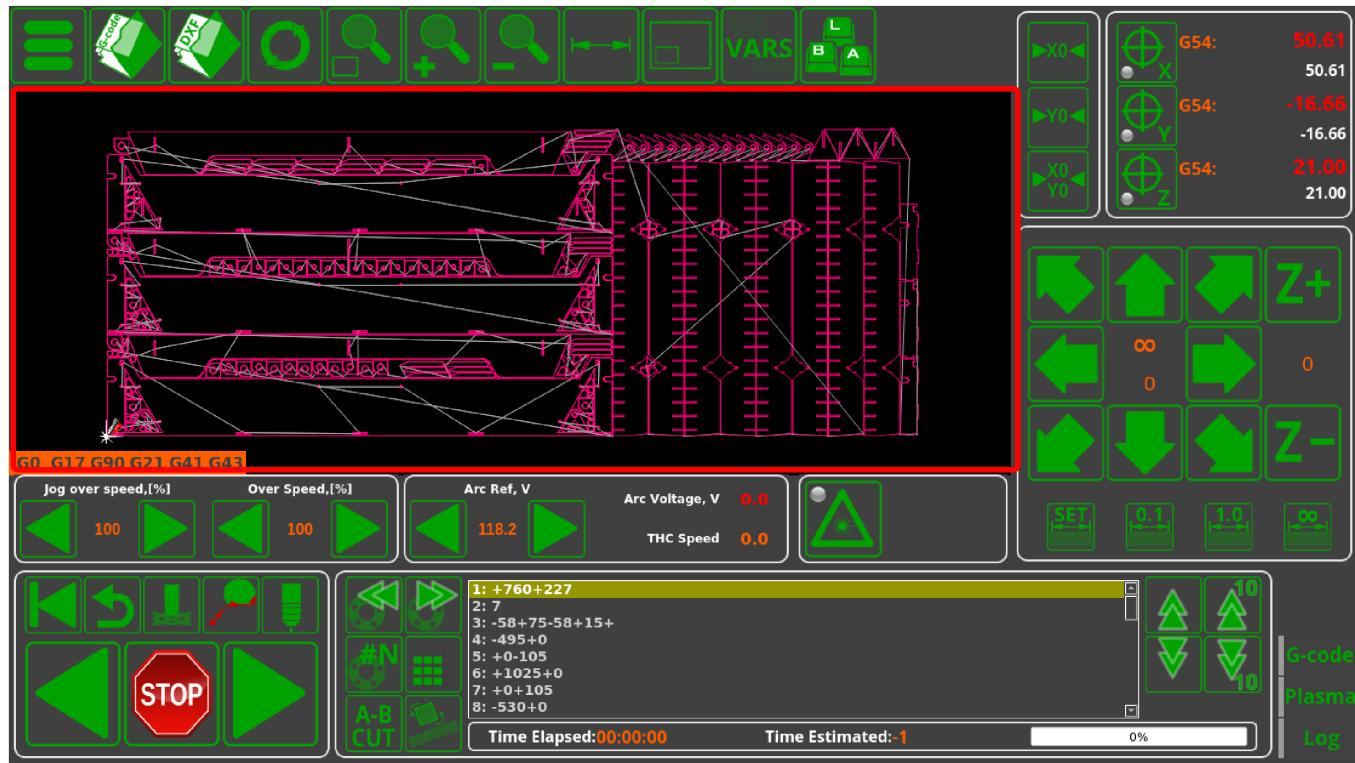
NCView is the 2D visualization widget to display an image of the imported G-code file such as the main visualization window in the 1366P profile (as a 3D visualization is unnecessary for a plasma/gas profile which will be doing all the cutting in the XY plane only).
