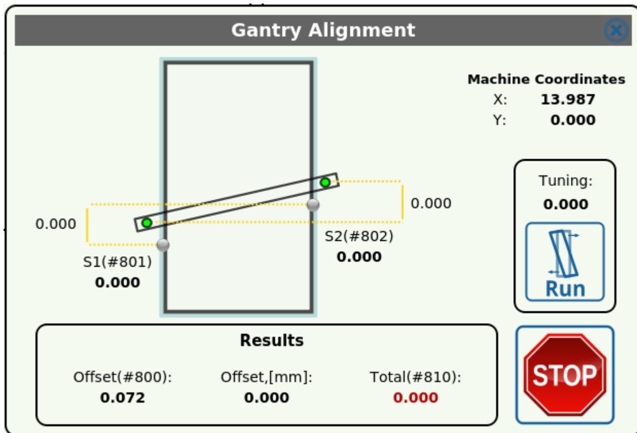
The background of the widget consists of a diagram of the machine. This diagram is embedded using the **skin** parameter.
