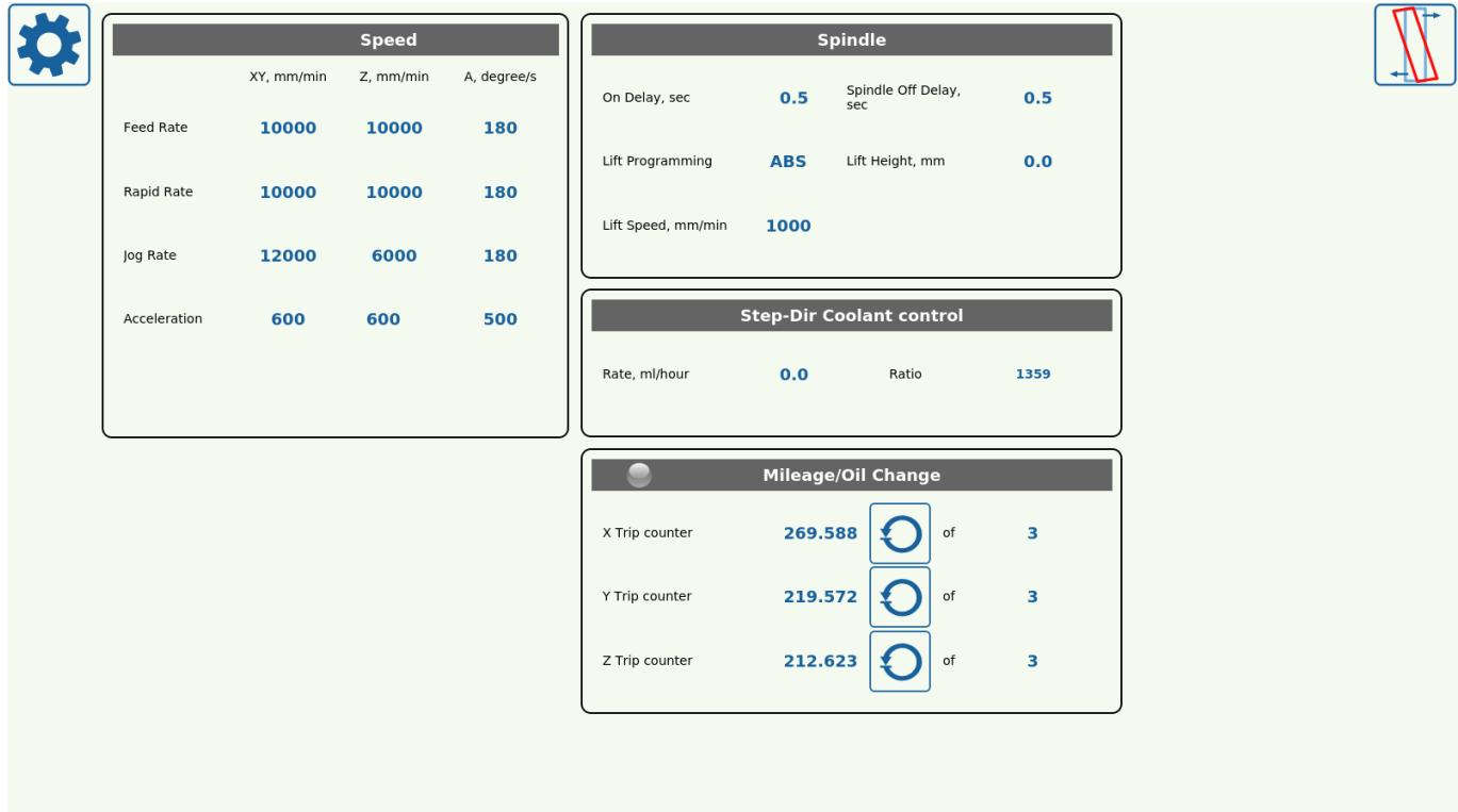
The rates are set in mm/min, and are useful if the hardware setup requires a different feed rate for cutting versus a rapid rate used primarily for movement. The values set here are default values for G0 and G1/G2/G3 and can also be changed through setting the speed to an Fxxx value manually either in the MDI mode or in the G Code program that the machine will be executing.
