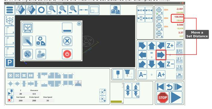
3. Measure the new physical position of the machine and record the distance actually physically traveled.
