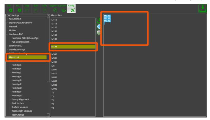
In case Gantry alignment procedure used instead of standard homing procedure, it might have different macro file name to not be mixed-up with standard homing procedure. For example - homing Y is "M132", gantry alignment is "M1321". This is just example, any of macro filename can be choosen. The result of Home-All macro would be
