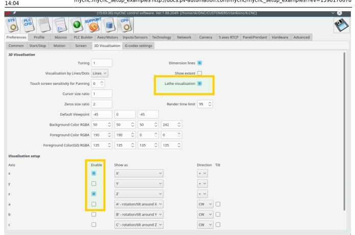
4. Check G-code settings related to Lathe operations in **Cfg** - **Preferences** - **G-codes settings** configuration dialog
