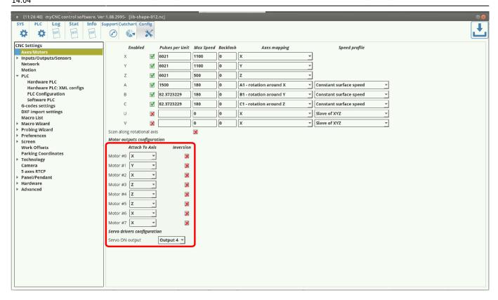
In the same window, the general calibration for the pulses per unit can be performed. This is done in order to calibrate the software readings of the machine (how much the machine "thinks" it has moved) versus the actual physical movements of the machine (how much it has actually moved). To do that:
