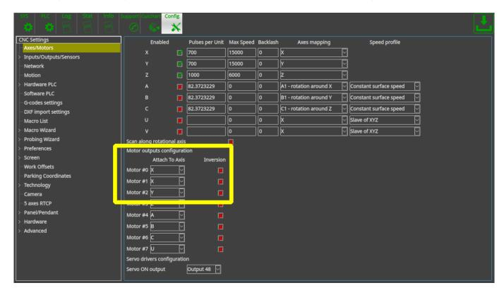
Next picture shows how to attach the Y axis to motor outputs #1, #2.
