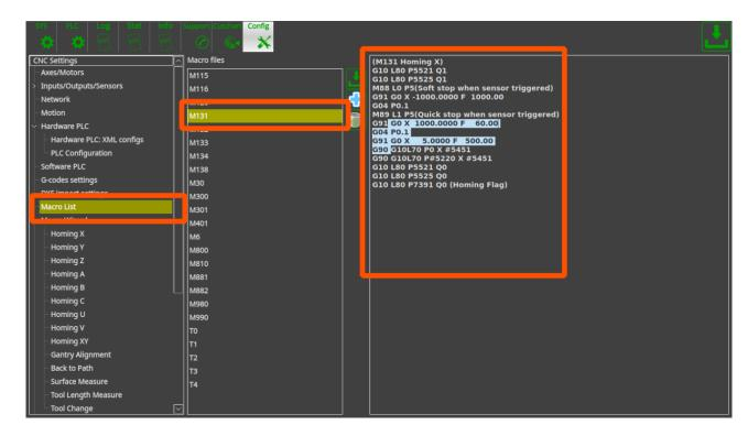
Home-All macro M138 is a simple macro file which runs in series macro files for all axes. For simple 3 axes machine it would be like this
