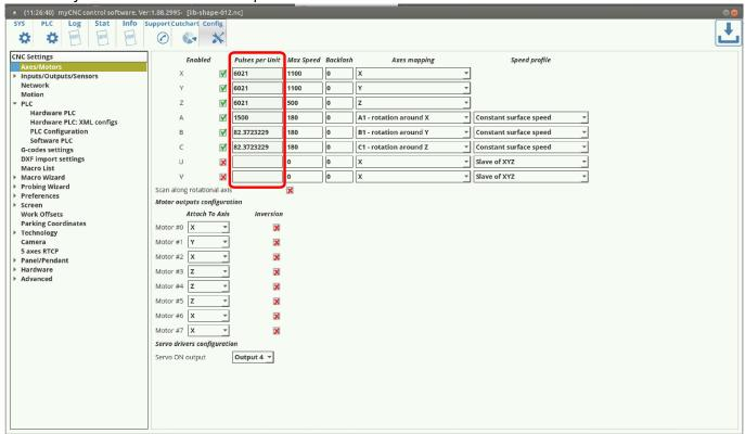
6. Input the new number of pulses per unit into the software.
