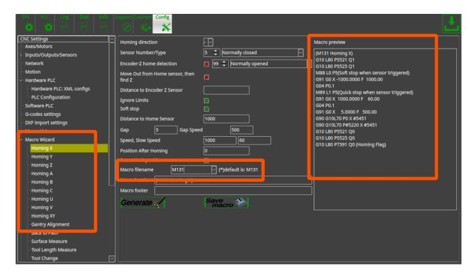
By using the macro wizard you just point homing moving direction, input number used for home sensor, sensor type (normally opened/closed), homing and probing speed, parameters of Encoder Z-label (if used to find precise homing position) and some other parameters. Macro file will be generated on the widget "Macro preview" by pressing "Generate" button. If the macro is ok, the button "Save macro" should be pressed to save macro file on a storage device (HDD, SD
