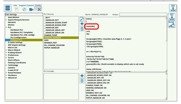
Note that the axes for which the homing is not required (Axis C in this case) have also been commented out. If only select axes need to be included in the homing procedure after the emergency stop, these can be configured in the code by adding/deleting forward slashes in front of the respective axes' commands.
