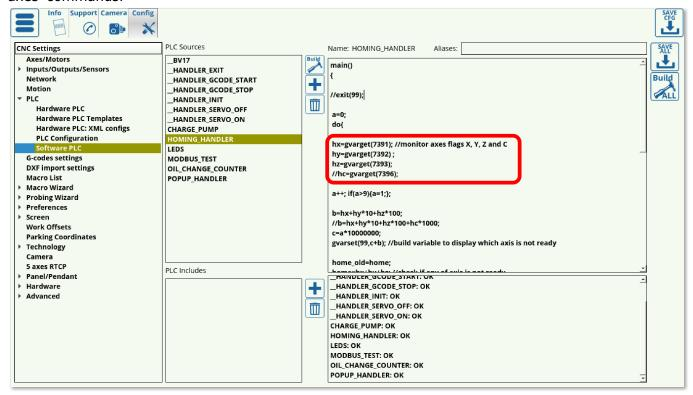
At this point, in an emergency stop situation, myCNC will prompt the user to run the homing procedure for the selected axes before any other action is taken after starting the machine back up again.
