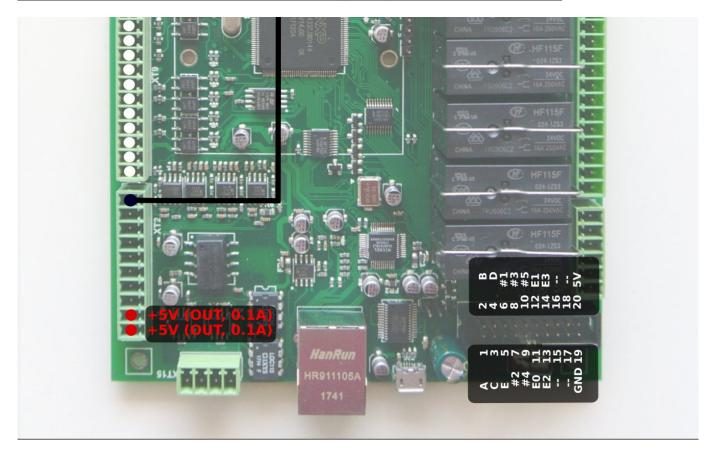
These pins are actually Binary inputs #16, #17, #18, #19 which are permanently configured as Encoder#0 and Encoder#1 in myCNC-ET7 controller firmware. This is the reason Slow Encoders #0, #1 configuration for ET7 controller in myCNC software is ignored and can be skipped. However, Encoder #2, Encoder#3 can be attached to any or binary inputs and configured accordingly.
