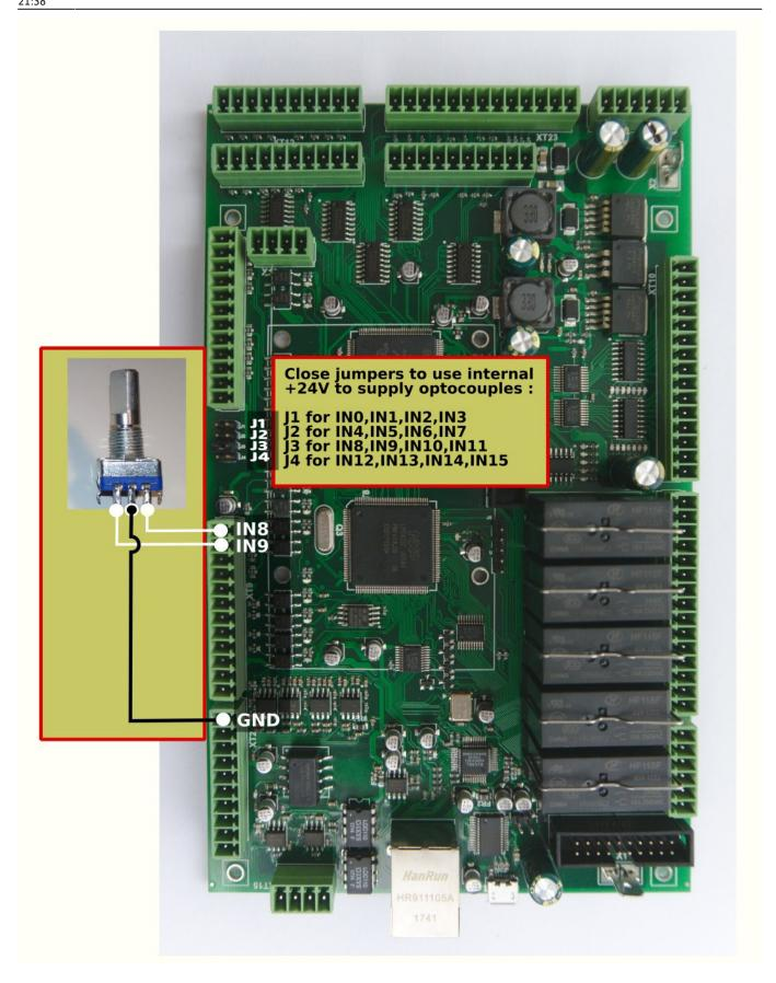
Encoder should be setup in **Cfg→Inputs/Sensors→MPG through binary inputs** configuration dialog.
