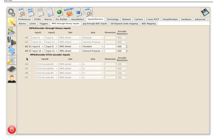
There are 2 encoders attached on Inputs #8,9,10,11 and set up in the dialog.
