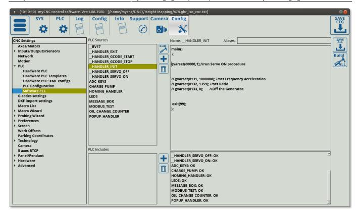
As can be seen, writing 1 to the register 60000 will turn the PIDs on, while writing 1 to register 60001 will turn the servo PIDs off. This will also be used in manual servo control, where a button can be utilized to quickly switch the motor on and off.
