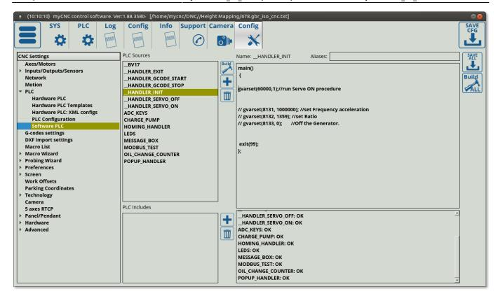
As can be seen, writing 1 to the register 60000 will turn the PIDs on, while writing 1 to register 60001 will turn the servo PIDs off. This will also be used in manual servo control, where an on-screen button can be utilized to quickly switch the motor on and off.
