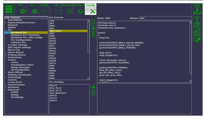
If the Stop button is pressed TWICE, the OFF.plc procedure will be used (the OFF.plc command is also launched upon completion of every small command, including macros and single G-codes completion). Below is the default code for the OFF.plc procedure for the X1366P profile (note that the procedures will be different for other profiles and different user cases):
