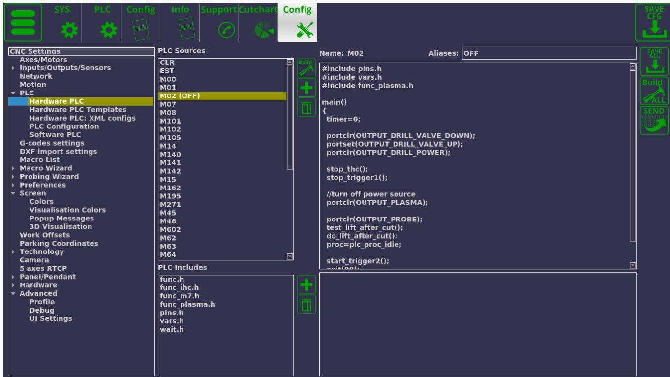
If the Stop button is pressed TWICE, the OFF.plc procedure will be used (the OFF.plc command is also launched upon completion of every small command, including macros and single G-codes completion). Below is the default code for the OFF.plc procedure for the X1366P profile (note that the procedures will be different for other profiles and different user cases):
