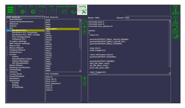
If the Stop button is pressed TWICE, the OFF.plc procedure will be used. Below is the default code for the OFF.plc procedure for the X1366P profile (note that the procedures will be different for other profiles and different user cases):
