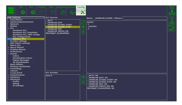
As can be seen from the code above code, in its default configuration the handler will simply activate and then close, not performing any additional actions. However, in situations where it is necessary to add a command which will activate whenever the G-code run has stopped, \_\_HANDLER\_GCODE\_STOP can be altered. For example, the code can be changed to look the following way if it is necessary, for example, to turn off the output port #3 whenever the run is stopped:
