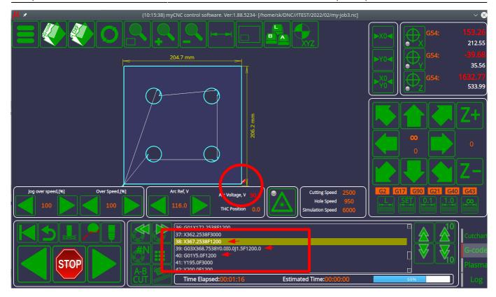
As can be noted from the Path Rules, the example above will have a speed reduction to 40% of the original speed at the arcs on each of the part's corners.
