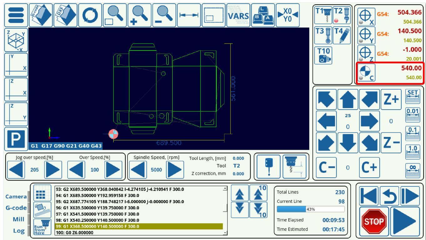
The M212 PLC exists to remove this positive/negative degree turn that is larger than 360 degrees at the program start. This is useful if the user wants to stop the knife from spinning back multiple times to its 0 position on the c-axis as the program is starting (however, this will still allow the knife to rotate an angle less than a full revolution in order to align itself properly).
