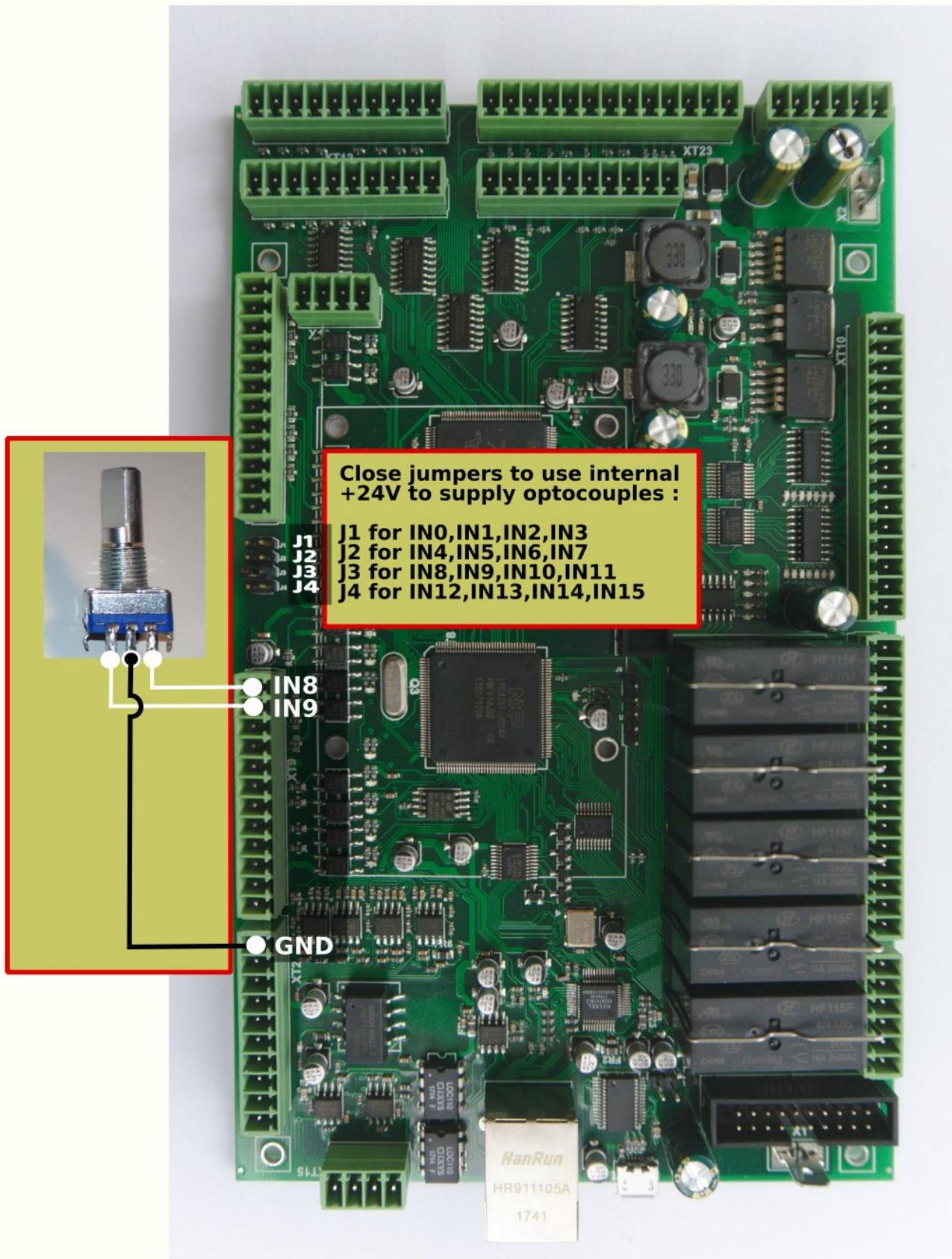
Encoder should be set up in the **Config > Inputs/Outputs/Sensors > MPG through binary inputs** configuration dialog.
