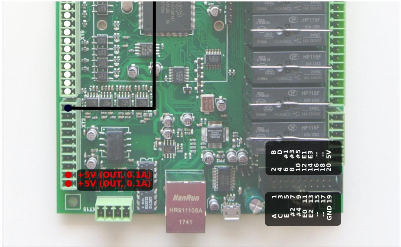
These pins are actually Binary inputs #16, #17, #18, #19 which are permanently configured as Encoder#0 and Encoder#1 in myCNC-ET7 controller firmware. This is the reason Slow Encoders #0, #1 configuration for ET7 controller in myCNC software is ignored and can be skipped. **However, Encoder #2, Encoder#3 can be attached to any or binary inputs and configured accordingly when using the ET7 board.**
