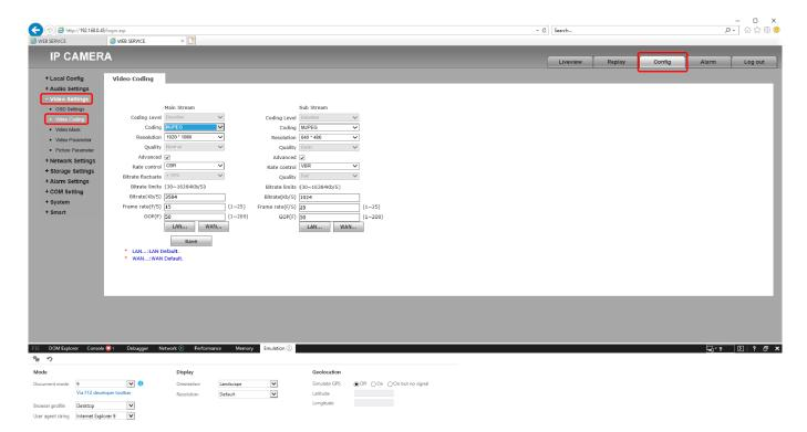
• In the Video Coding window, check that the Coding field is set to MJPEG for best image recognition results when using the myCNC Vision System. Here you can also change the resolution and the frame rate of the camera. Typically, a frame rate of around 10 frames/sec is sufficient for the myCNC Vision System. Click 'Save' once you've successfully altered the necessary settings:
