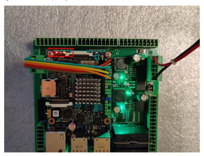
If the SD card is not plugged in and the computer is not booting up, only the RED light will be on, as shown in the image below:
