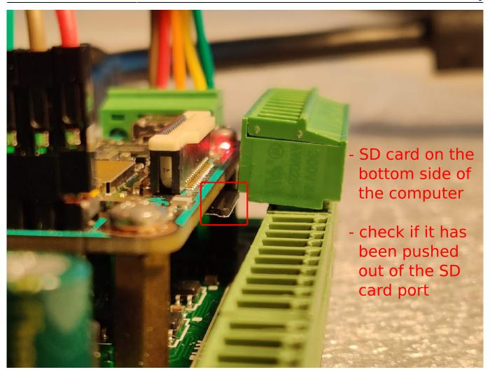
In order to fix this issue, it is recommended to plug in the connectors at a slight angle, monitoring the SD card as the connectors are put into place. This will prevent the SD card from popping out, and the boot up process will proceed as normal.
