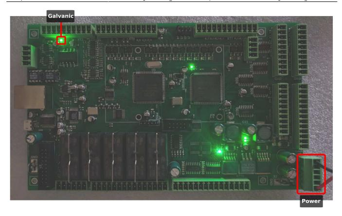
• Two LEDs near the processors should also light up, one solid and one blinking at about 1 blink per second. This signifies that the processors are functional:
