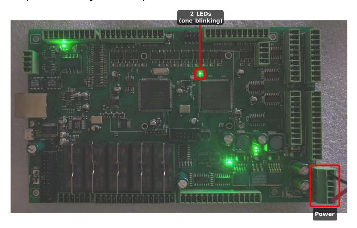
Overall, 6 LEDs should light up after supplying power to the board.
