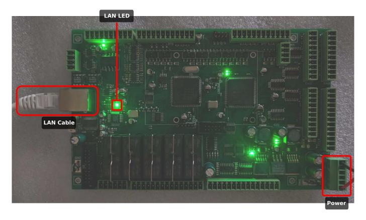
Overall, 7 LEDs (with one of them blinking) should be light up at this point.
