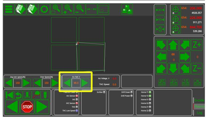
In Settings > Config > Technology > THC, check that the Alarm Arc Voltage Difference and Alarm Arc Voltage Rise aren't set to a value that's too low - in cases where the difference between reference and measured voltage is too great, a small value of the Alarm Arc Voltage Difference will prevent the THC system from starting. Set the value to 1000 to temporarily disable this feature.
