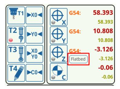
This button toggles the display of the Z-axis coordinate with/without the flatbed correction.
