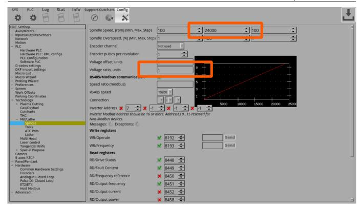
At this spindle speed, a full 10V signal must be sent to the analog output, so the "voltage ratio" coefficient is set to "1" (in the case of, for example, a spindle with an input signal range of 0-5V, this coefficient would be 0.5 to get a 5V signal at maximum speed).
