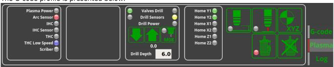
This screen presents the user with the options and indicators for the plasma controls. The five buttons on the right side of the tab are the most commonly used:
