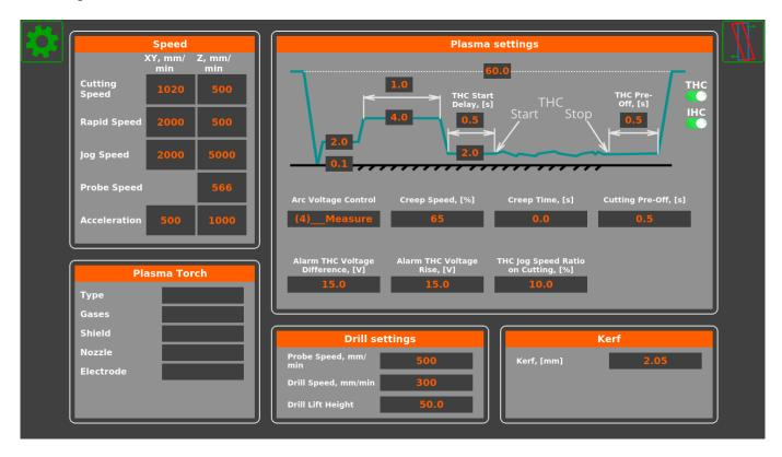
This settings window allows to specify the distances within the plasma cutting cycle, as well as functions such as THC and IHC. It also serves as the quick settings window which is always accessible to the operator, as opposed to the general settings, which might be open or closed to the operator
