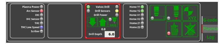
The homing sensors LED show two sensors per the X, Y and Z axes. Not all of these sensors are commonly used during the homing procedure on different machine setups, so the user is free to edit the x-plasma.xml file in the X1366P profile folder to not display the unnecessary LEDs:
