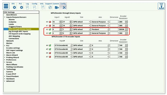
There are 2 encoders attached on Inputs #0,1,2,3 and set up in the dialog.
