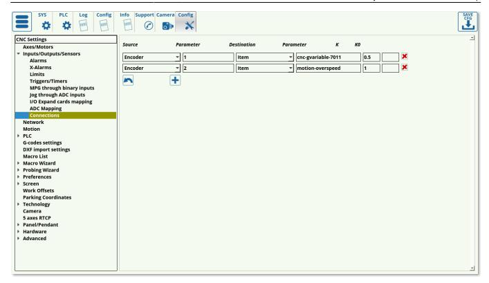
A general purpose encoder can be connected to one of the system variables for convenient control.
