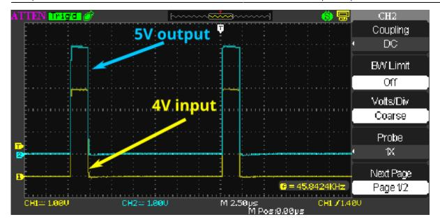
The ClearPath driver manual provides an explanation as to why their drivers are not directly compatible with 5V differential outputs, such as the ones used on the myCNC controller boards:
