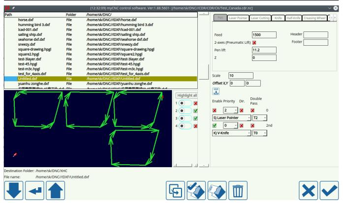
In the examples above, two contours are selected to be cut clockwise, while two are selected as counterclockwise.
