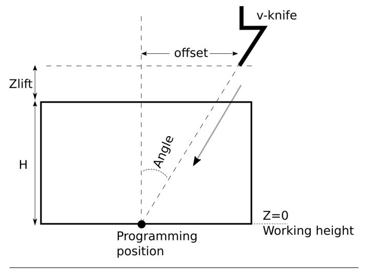
In the diagram above, the working height is the cutting height. The entry is made at H, the material thickness, plus the lift height.
